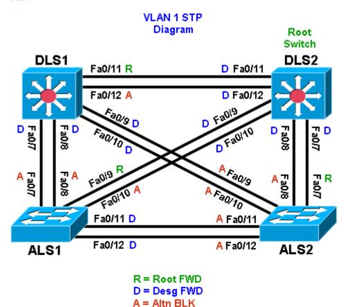
In this lab, the default operation of IEEE 802.1D spanning tree was observed. Since no bridge priorities were specified, the switch with the lowest MAC address was elected as the root. The link providing the lowest root path cost was chosen as the active link. If costs were equal, the tie was broken first by the lowest sender BID of the BPDU, then by the lowest sending port priority and last by the lowest sending port number.
