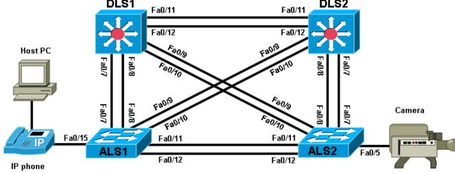
All Switch-to-Switch Connections Are 802.10 trunks
